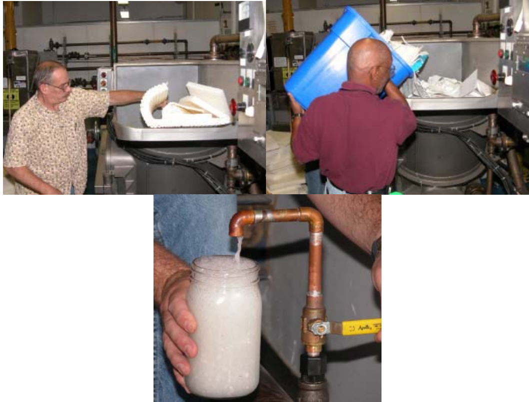
Figure 3. Feeding Green Cell Foam and Paper Into Large Pulper, and Taking Sample from Discharge Port
